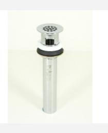
All Brass Lavatory Grid Drain, with overflow, with 6" Length / 17ga. Tailpiece. Forged brass face features concave design for positive drainage leaving little standing water.
