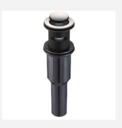
Push and Lock (clicker) Sink Drain, Polished 304 Stainless Steel clad top and plunger. Fits sinks with and without overflow. 6" Long plastic tailpiece, comes complete with lift rod and linkage. Converts to a grid drain using (10286) 600CL11.
