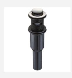
Push and Lock (clicker) Sink Drain, Polished 304 Stainless Steel clad top and plunger. Fits sinks with and without overflow. 6" Long plastic tailpiece. Converts to a grid drain using (10286) 600CL11.
