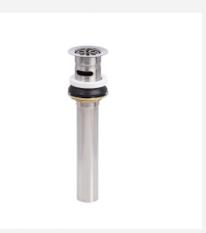
Polished 304 Stainless Steel Grid Drain with overflow holes and 6" tailpiece. Converts to clicker by replacing the grid insert with a clicker stopper (7800-1).
