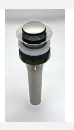
Polished 304 stainless steel Push & Lock (clicker) pop up drain Sink Drain with overflow holes and 6" tailpiece. Converts to grid drain by replacing the clicker stopper using a grid insert (10286 - 600CL11).
