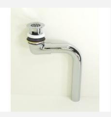
All brass, chrome plated, Sink or Lavatory Grid Drain, with Offset tailpiece for wheelchair accessibility. Forged brass face features concave design for positive drainage leaving little standing water. See each listing for face and overflow variations.
