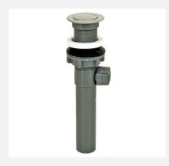
Plastic Sink Drain single piece Pop Up Drain without Overflow Easy Assembly with with Stainless Steel clad waste seat and plunger, comes complete with lift rod and linkage.
