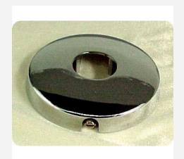
Diecast, flange with set screw. 7/8" ID for 1/2" nominal pipe size. Smaller ID 13/16" fits snugly on shower arms.
