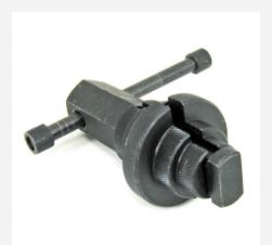
Spud Chuck (Nipple Extractor) with 1" to 2" Capacity. Expands with eccentric action of twin jaws with knurled gripping faces.
