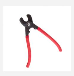
Heavy Duty Wire Cable Cutter. For Copper and Aluminum only. Cuts up to 3/4" diameter. Heat treated cutting edge.
