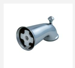
6" Long zinc tub spout with Luxury Design, Slip Fit 5/8" OD copper tube, and Front Diverter
