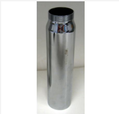
Brass tailpiece converts standard grid drain from 1 1/4" x 1 1/2". 6" 17 Gauge.
